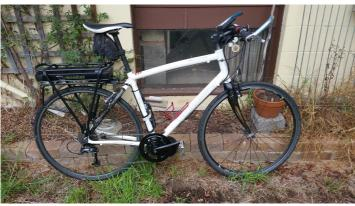
Enthused by the current trend for ebikes, I have electrified my old(ish) Specialized Pro. An aluminium frame-bike of around 11kg. The motor is a Bafang 250w powered by juice from a 19.2ah battery. The system has a technology from RevBikes called lovo (low voltage) which precludes overcharging, but lowers the top ah to 18. This much improves battery life. Only had a few rides, but I am very pleased that I can now negotiate the mountains of Eltham better. Allan G
